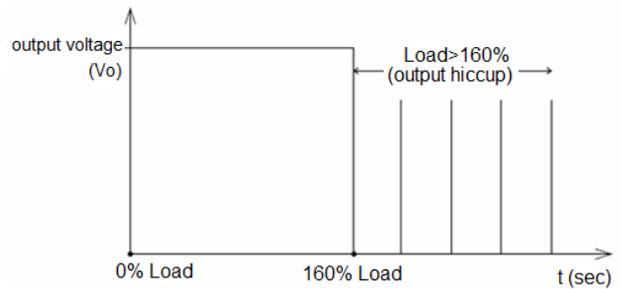
Additionally, if the 48 Volts' lout is  $>100\%$ ; but  $<160\%$  for a prolonged period of time (depending on the load), the Over Temperature Protection (OTP) will be activated due to high temperature on critical components. The power supply will then go into latch mode.
